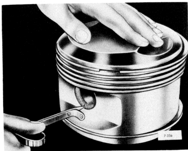
Figure 117—Removing Piston Pin Retainer
