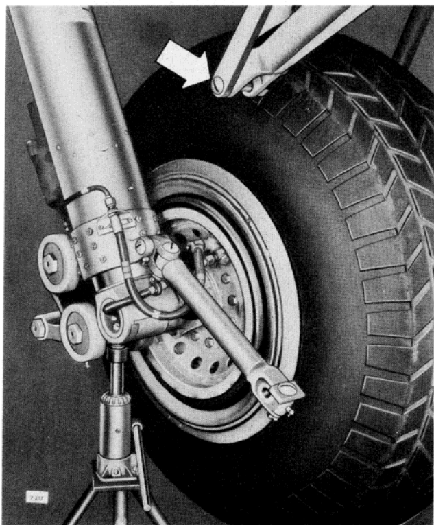
Figure 94—Drag Link Disconnected
