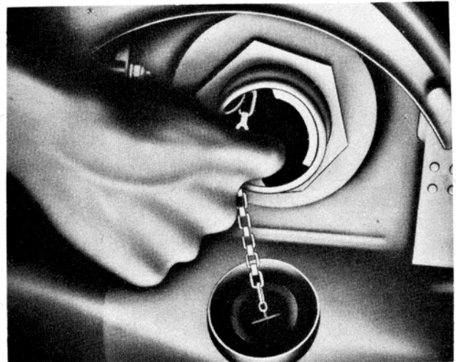
Figure 32—Replenishing Test—Supercharger Oil Tank
