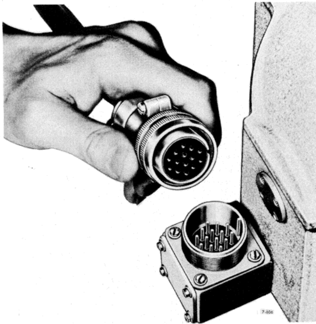
Figure 262—Slot on Plug Must Mate with Key on Receptacle Sleeve
